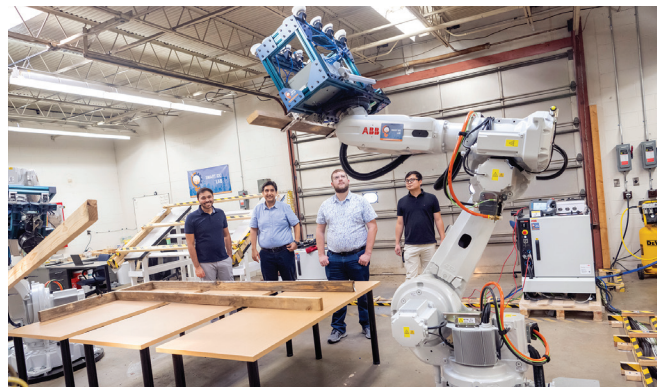
Faculty and students in UF's College of Design, Construction and Planning are programming large robotics for construction framing, equating to cost savings in the building industry.
